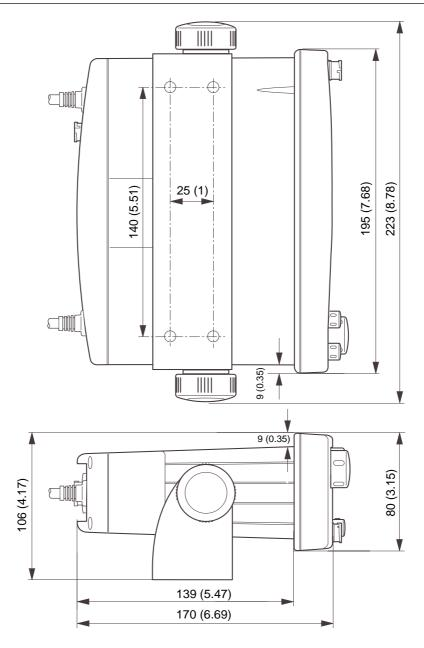
Figure 2-2 Outline and Mounting Dimensions All dimensions are shown in millimeters and (inches)
